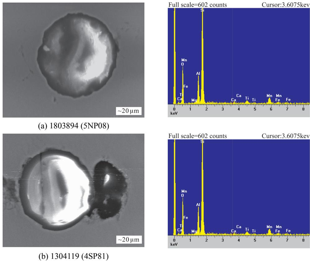
**Fig.2.** Inclusion shape and composition of 50CS1300 with high core loss.
