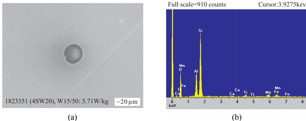
**Fig.1.** Inclusion shape and composition of 50CS1300 with low core loss.
