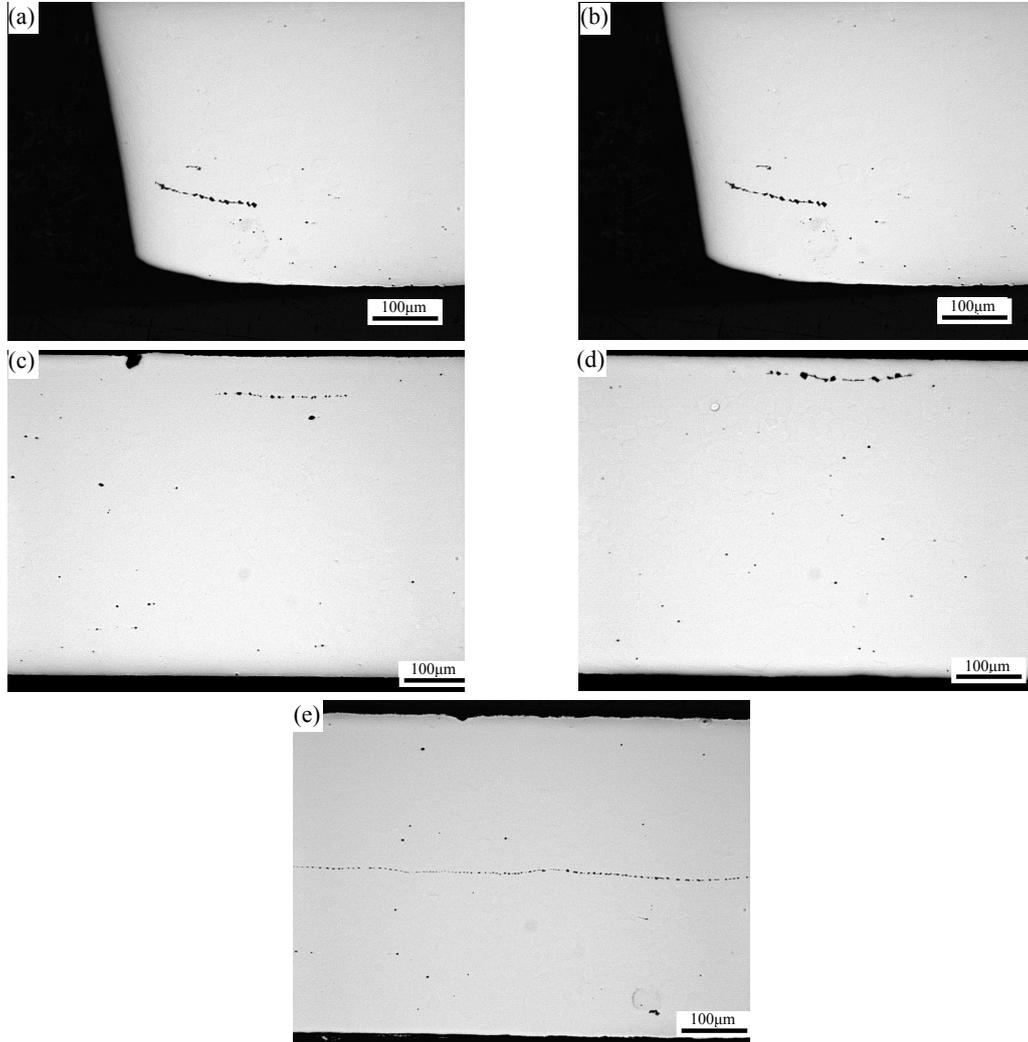
**Fig.3.** Inclusion shape of 50CS1300 with high core loss. (Corresponding to Table 1)
