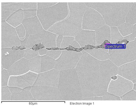
**Fig.4.** Inclusions broken into small pieces with a long chain.
